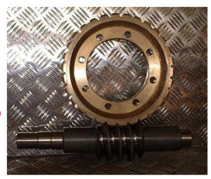
This system guarantees maximum operational safety. If compared to others types of reduction unit - such as ordinary reduction gears or epicyclical gears -, the advantage of our bronze worm wheel and worm screw system is that it IS NEVER SUBJECT TO ACCIDENTAL REVERSE MOTION.
